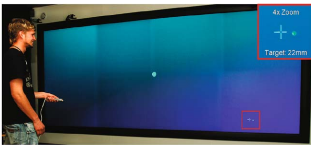
Fig. 12 Laser Pointer Interaction in front of a large high-resolution display. Squidy facilitated the integration and evaluation of precision enhancing and smoothing techniques, allowing the precise selection of targets as small as 22 mm in diameter from a 3 m distance [21]
