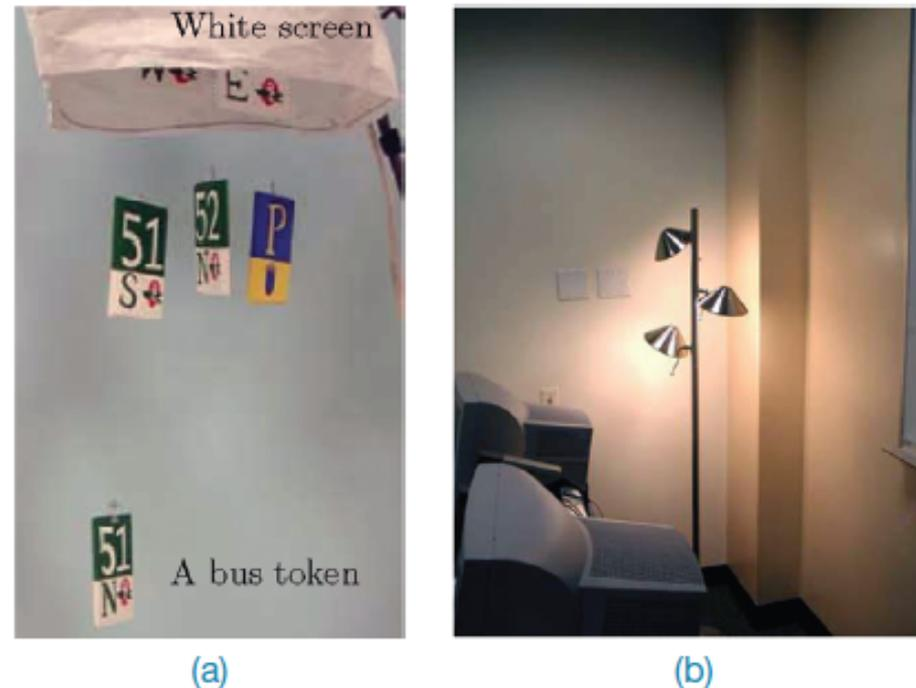
**Figure 15.2** Two ambient devices: (a) bus indicator, (b) lightness and darkness indicator
