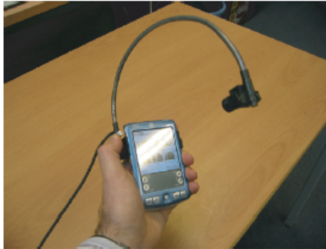
Figure 14.4 The Tracksys system being used with a mobile device camera that attaches to a flexible arm, which mounts on a mobile device, and is tethered to the lab
