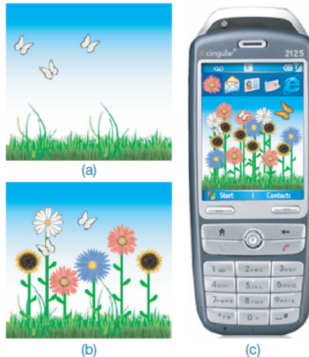
Figure 14.8 UbiFit Garden's glanceable display: (a) at the beginning of the week (small butterflies indicate recent goal attainments; the absence of flowers means no activity this week); (b) a garden with workout variety; (c) the display on a mobile phone (the large butterfly indicates this week's goal was met)
