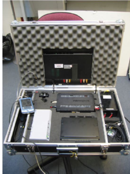
Figure 14.3 The Tracksys lab-in-a-box system, which comprises components that pack into a heavy duty padded flight case plus a PC system
