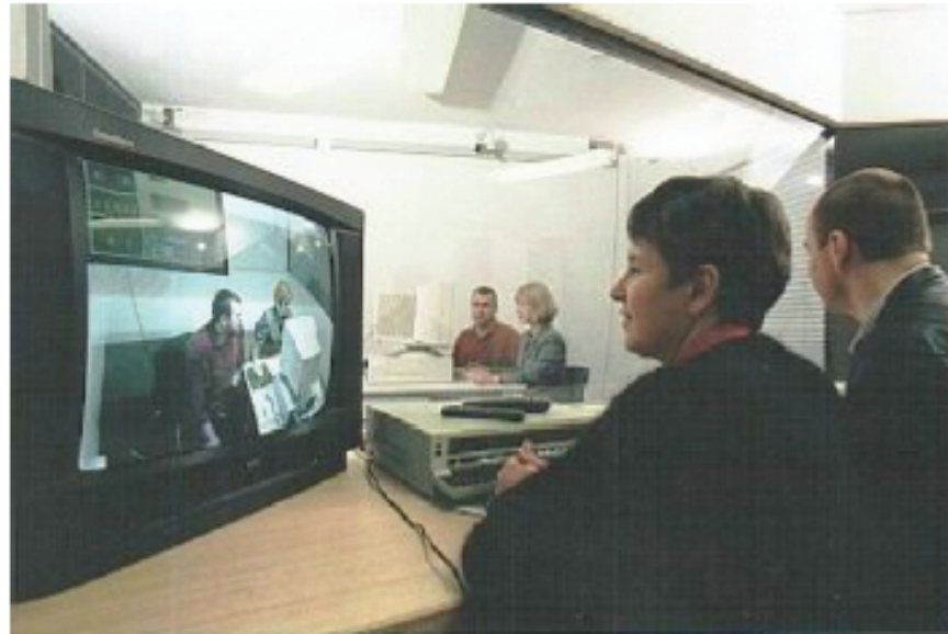
Figure 14.1 A usability laboratory in which evaluators watch participants on a monitor and through a one-way mirror
