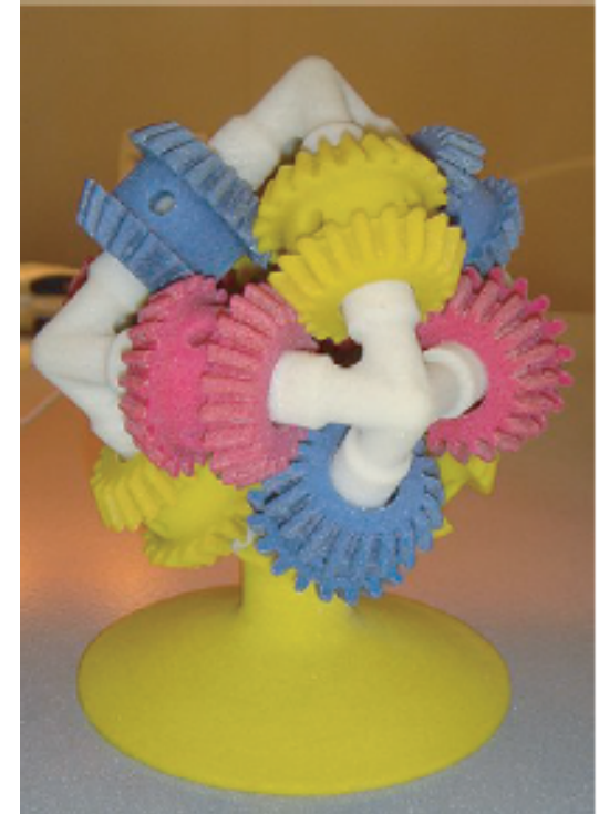
Figure 11.1 (a) Color output from a 3D printer: all the gears and rods in this model were 'printed' in one pass from bottom to top, and when one gear is turned, the others turn too. (a)
